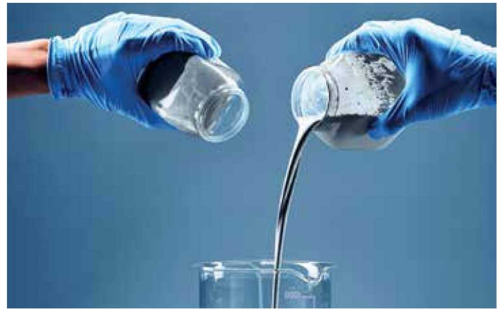
Left: Pigment preparation without dispersing agent. Right: Pigment preparation with 0.1% POLYRON® N. Adding just 0.1% POLYRON® N, the viscosity can be strongly reduced at the same PVC, thus a flowable paint can be achieved.
